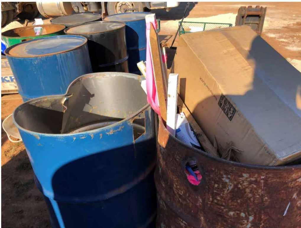
Photograph 15: 200L drums with holes cut for lifting points – sharp edges evident and pose a risk
